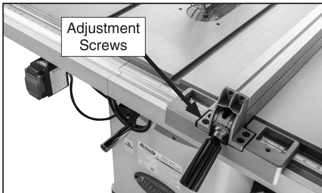
Figure 125. Location of adjustment screws for setting fence parallelism.
